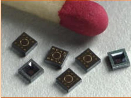
Infineon will provide its semiconductor and MEMS expertise to the Hosiden which develops and produces microphones for cellphones, notebook PCs, digital still cameras and automotive navigation systems. Hosiden intends to benefit from the MEMS technology in that MEMS-based microphones are smaller and more rugged than conventional types.
