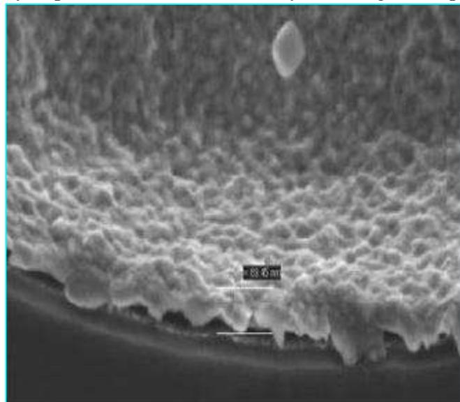
The feasibility of the process was demonstrated with a 5- $\mu\text{m}$ -wide, 25- $\mu\text{m}$ -deep via, with a TiN barrier layer deposited in collaboration with IMEC. As shown in the photo, the conformal copper layer at the bottom of the via is ~50 nm thick. Process time was 5 min.
