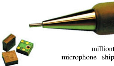
**Microphones - Akustica** pioneered system-on-chip acoustic systems by combining on-board electronics with MEMS microphones on the same chip. Everyone else uses a 2-chip system [as far as I know]. They shipped their two-millionth digital microphone. Akustica's two-millionth microphone shipped just three months after its one-millionth
