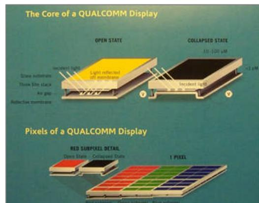
Many others MOEMS systems use mirrors that can tilt (TI's DLP) or be steered; 3-axis. The QUALCOMM displays are designed to enhance the hand-held products by providing more run-time per charge and expanding the capabilities of today's mobile devices. Their MEMS displays will be available in Hisense mobile phones in 2008. Source: Tech On
