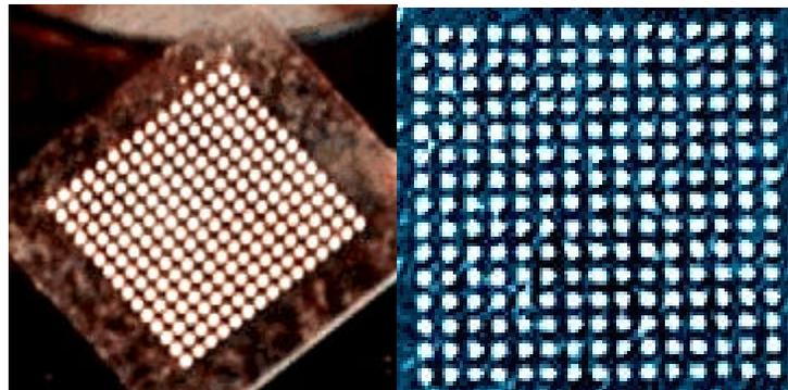
**FIG.1 - Grid Array Z-Axis Adhesive (Cookson Electronics)**
