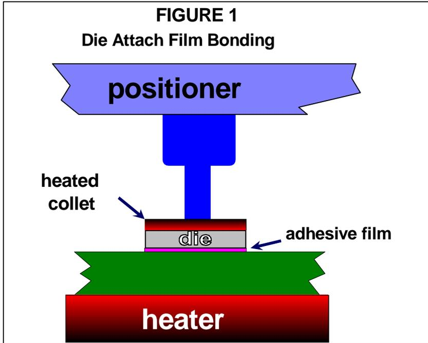
low as 100°C and up to over 300°C. Bonding limits fall between the glass transition temperature ( $T_g$ ) of the polymer and the decomposition point. Applied pressure forces the softened or liquefied polymer into the surface microstructure of the adherends, producing a mechanical link. The time factor, or dwell, allows heat to distribute at the interface and the fluid polymer to penetrate the surface microstructures.
