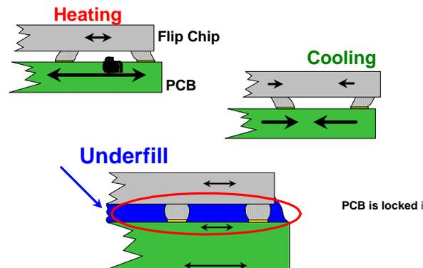
Figure 9. Underfill Locking Action
