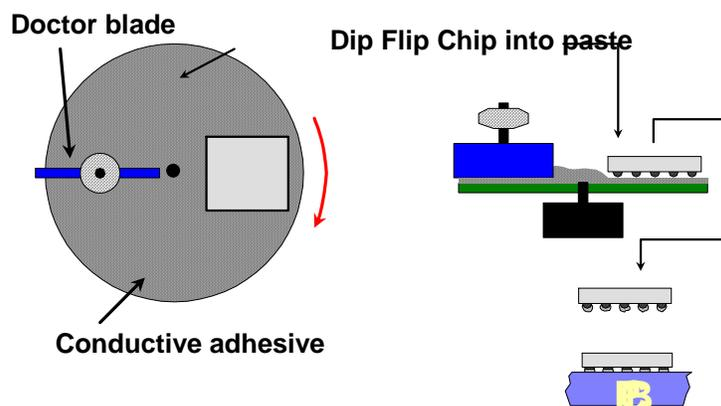
Figure 5. Polymer Dip Chip Process
