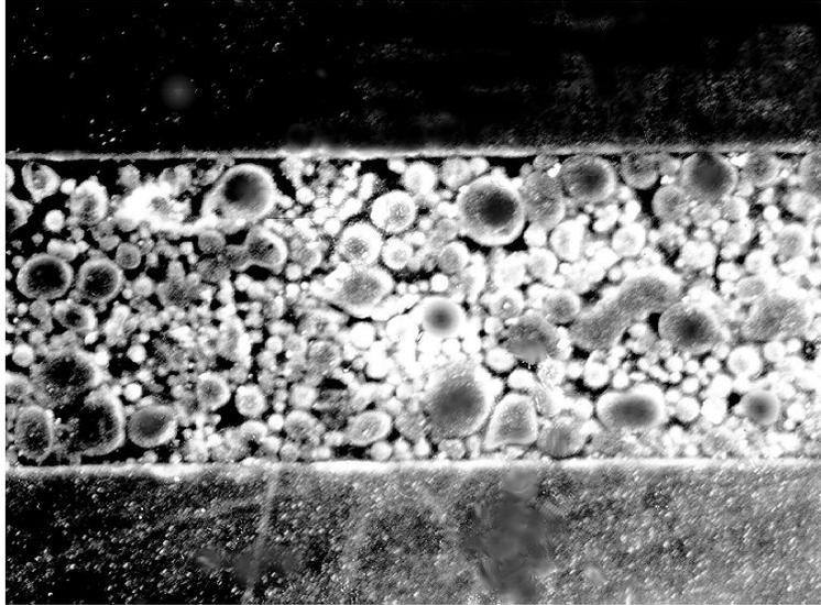
Figure 6. Underfill Cross Section
