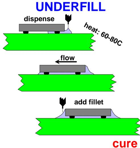
Figure 8. The Basic Underfill Process
