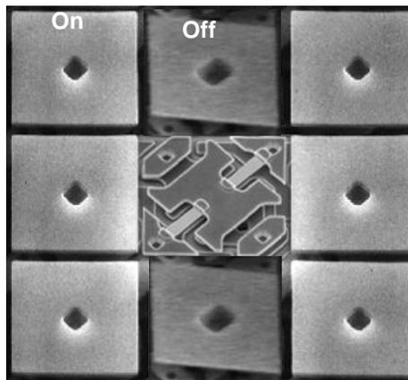
Figure 6 - DMD™ Structure – Texas Instruments [3]
