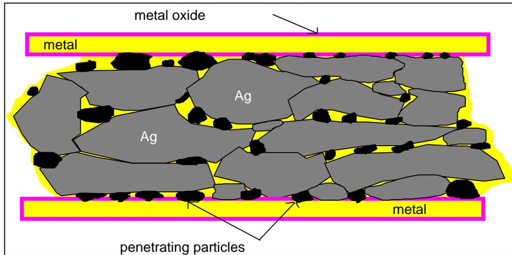
Although there is a small rise in resistance because of degradation of the copper at the edges of the adhesive junctions, the total increase is under 20%, the criterion set by AT&T. Of course, moving to a gold-plated PCB reduces even the small increase. These 1000 hour tests show even better stability than the Elektronik-Centralen study<sup>18</sup> after 168 hours 85%RH/85°C. Chart 1 shows the humidity aging results on untreated bare copper circuit boards with Sn/Pb-coated components.
