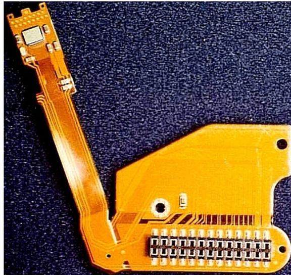
**Figure 9 – Disk Drive Flex with Flip Chip**
