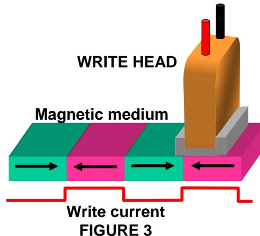
A timing clock is synchronized with disk rotation so that the location of the head with the magnetic “bit cells” is precisely known and controlled. Bits represent ones and zeros (reversed magnetic polarity). Although the disk is permanently magnetized, bits are easily reversed, or rewritten, as the head applies an opposite magnetic field produced by simply reversing the coil current. MR and GMR require more precise synchronization since the domains are smaller.
