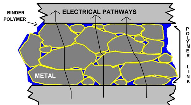
Although the adhesive should be viewed as an integrated system, this separation of mechanical and electrical properties provides advantages over solder, but also a few disadvantages. Since the electrical and mechanical performance can be independently modified, much more tailoring is possible than with solders. However, this independence also means that good mechanical performance
