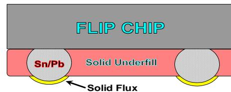
Figure 7 – Two-Layer Flux/Underfill
