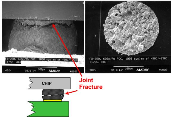
**Figure 1 – Fractured Joint**
