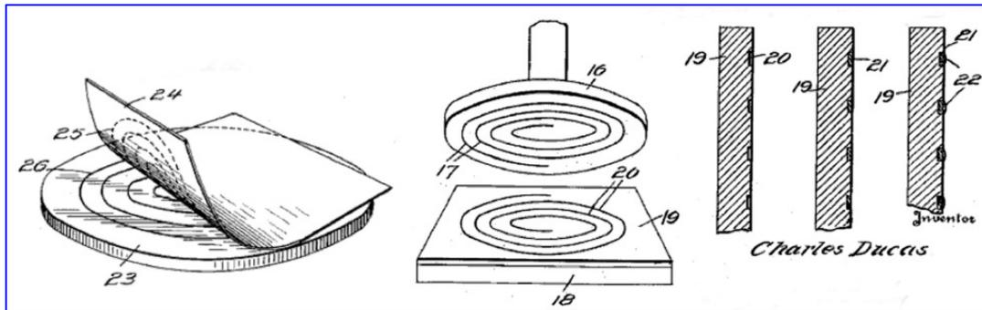
**Figure 1 - 1925 Groove & Fill Circuits; Reference 1**
