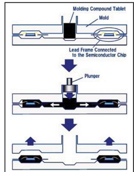
Figure 1C. Transfer Molding.
