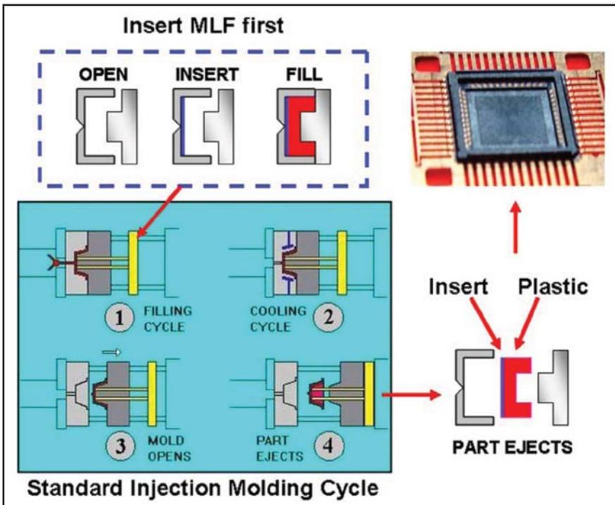
**Figure 2. Insert Molding Process.**
