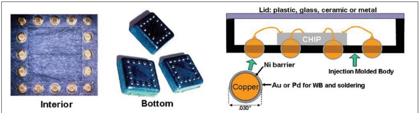
**Figure 4. Diagram: Low Ball Simplest Cavity Package.**
