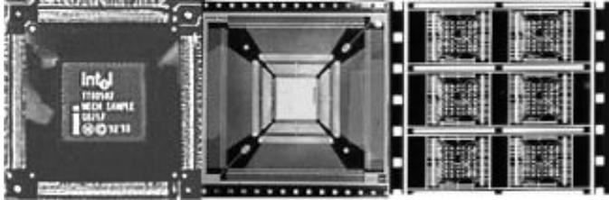
**Figure 8 - TCP and TAB = Flex Chip Carrier**
