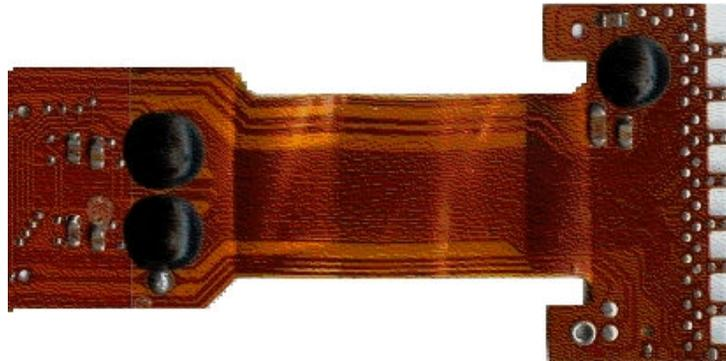
**Figure 8 – Flex HDD Circuit with COB**
