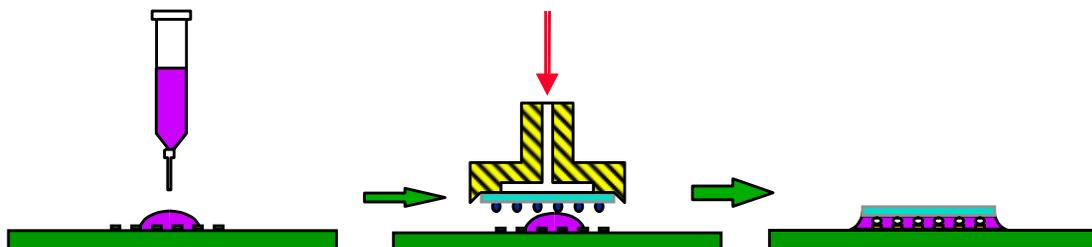
**Figure 10 – Pre-Applied Flux/Underfill Process**
