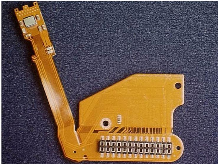
**Figure 9 – Disk Drive Flex with Flip Chip**
