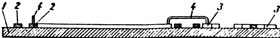
Figure 7 - Parolini Circuit with Jumper
