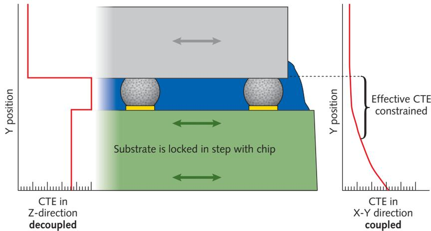
Figure 2. Underfill mechanism.
