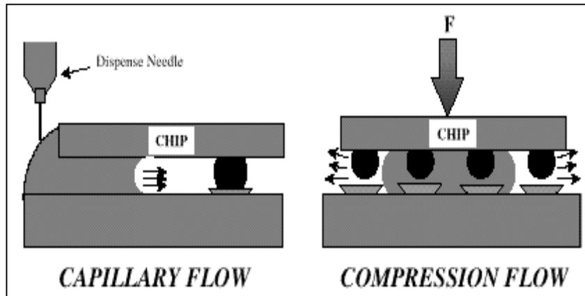
into the underfill unlike capillary underfills where the flow front displaces air. Figure 1 compares post-dispensed capillary flow to pre-dispensed no flow type of underfill.
