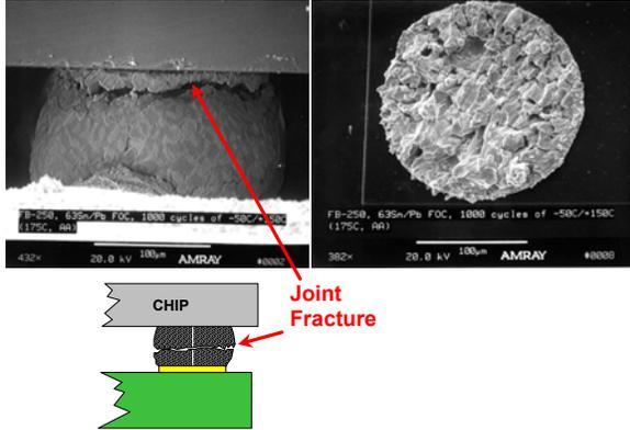
**Figure 1 – Fractured Joint**
