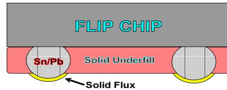
Figure 7 – Two-Layer Flux/Underfill
