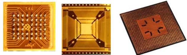
Figure 1 –  $\mu$ BGA, TAB and TBGA
