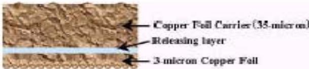
**Figure 2- Ultra-thin Copper on Carrier**
