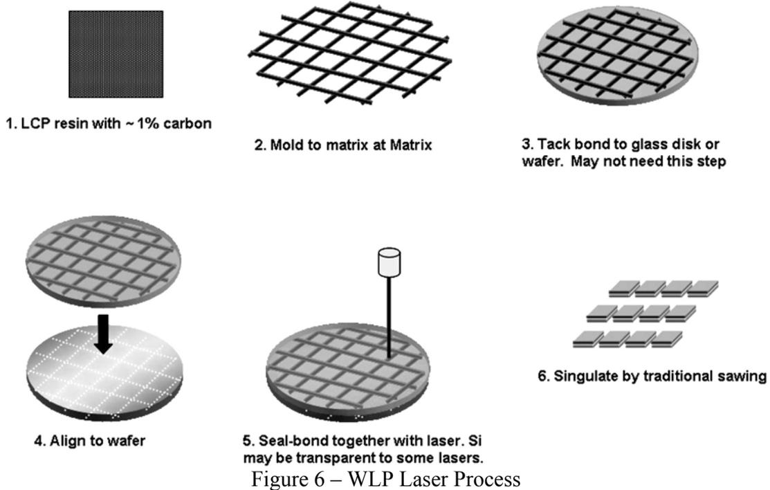
Figure 6 – WLP Laser Process
